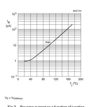
Reverse current as a function of junction Fig.7 temperature; maximum values.
